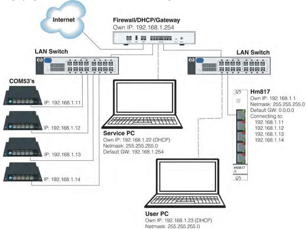
In this configuration, the internal LAN is used for communications between HM817/1 and COM53. All units are coded with a Static IP-address. In this configuration, all PC's within the network can get in contact with the IHM modules. Depending on the Firewall setting it may be possible to access the Internet from any PC in the network.
