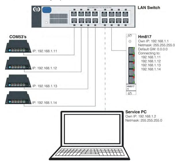
In this configuration, the network is solely used for communications between HM817/1 and COM53. All units are coded with a Static IP-address, no further equipment is required. In this configuration, there is no access from other networks. Also, the PC for configuration needs to be address coded when connected to the network.
