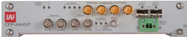
External ASI module for Phoenix C IDU, 4x BNC, 2x SFP ports with Time Synchronization
